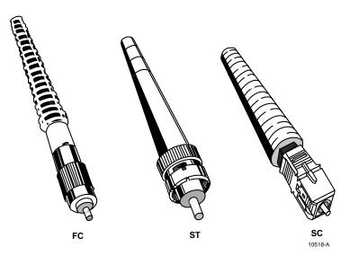
Figure 701-1. Optical Connector Identification
